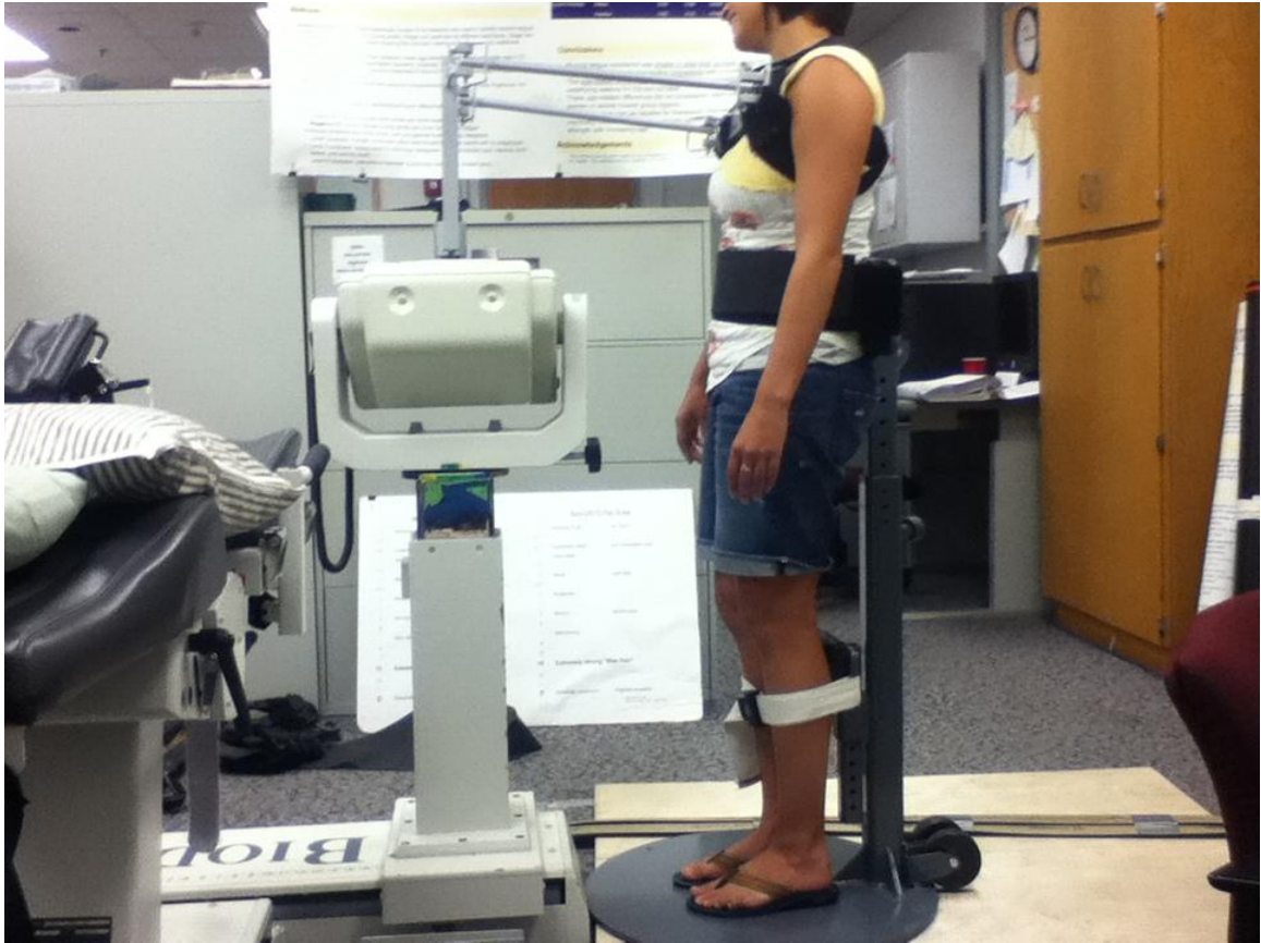
Figure 3 .3. Experimental setup for trunk rotational motion testing.
